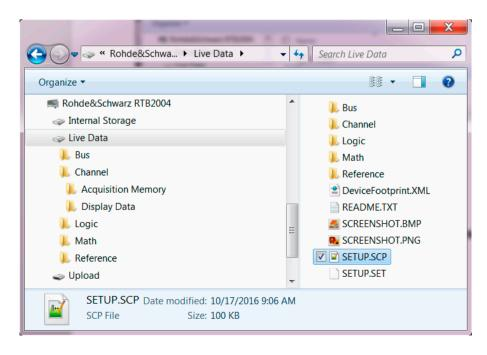
With the USB MTP implementation, easy access to live channel data and screenshots and integration into customers computing environment is possible
