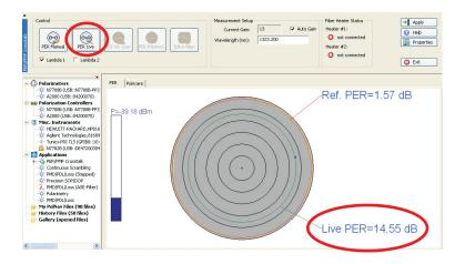
There are a number of options that can be used to influence certain aspects of the measurements. These can be configured in a dialog that can be accessed by pressing the **Properties** button, which is located at the right side of the application window in External PC mode and in the top button row of the application in Internal PC mode. Details on these options can be found in Application Properties on page 115.
