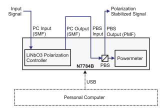
When it is set to **Analog In**, an appropriate external signal has to be provided and the N7784B will optimize the output SOP with respect to this feedback signal. Configure the N7784B according to the following setup:
