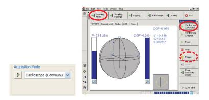
There are two options in this mode: Continuous and Oneshot. In the continuous mode, the measurement is restarted after receiving a trace. In oneshot mode the acquisition has to be manually (re)started by pressing the button next to the list box or by pressing **Trigger**, when using the Integrated PC Mode. To stop measuring in continuous mode select **Hold** from the drop-down menu or by pressing **Stop** respectively.
