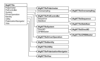
Figure 23 Diagram of COM/ActiveX-interface classes
